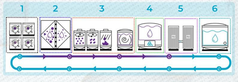
**Washing machines:** The set of industrial washing machines is connected through a common piping network that collects the used water from each washing machine and directs it to the ANHIDRA system for treatment.
