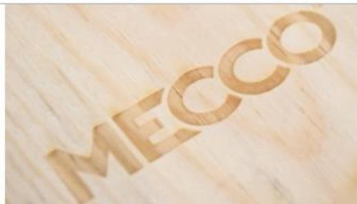
*CO2 Laser: Even absorption from a longer wavelength*
