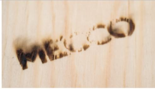
*Fiber Laser: Uncontrolled absorption effects from a short wavelength*
