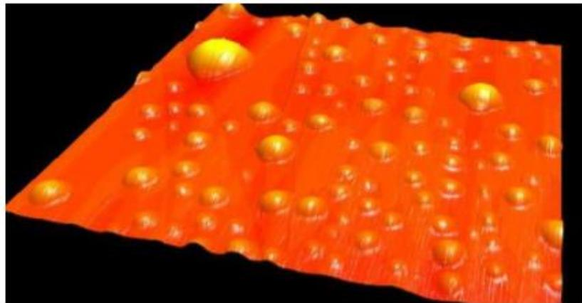
Nanobubbles at the interface between hydrophobic silica and water. Image credit: [Virginia Tech](#)
